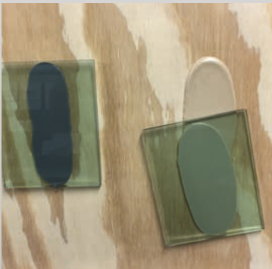
Picture of Sikaflex® Mirror Grip on left and Gunther Ultra Bond® on right. Slip down test 4 minutes after installation.
